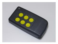
The Remote Control is powered by a Battery Type CR2032. To change the battery, use a crosshead screwdriver to remove the screw on the cover.
